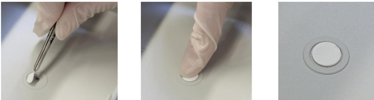
Figure 3: mounting of DAE D11
