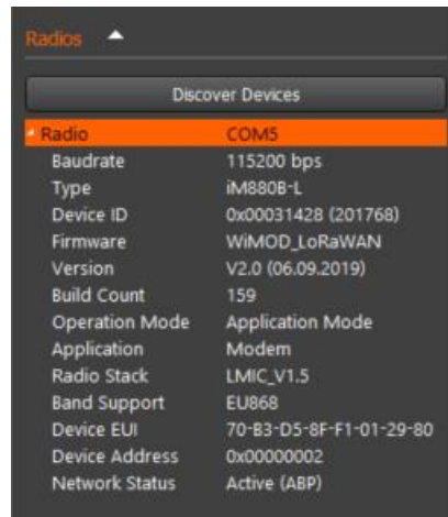
Figure 2-2: Connected iM880B on serial com port
