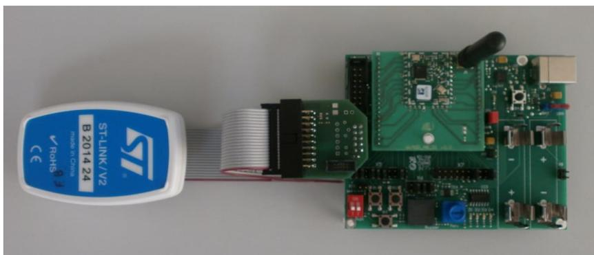
Fig. 2-1: ST Link V2 programmer
