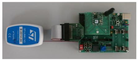
Fig. 2-1: ST Link V2 programmer
