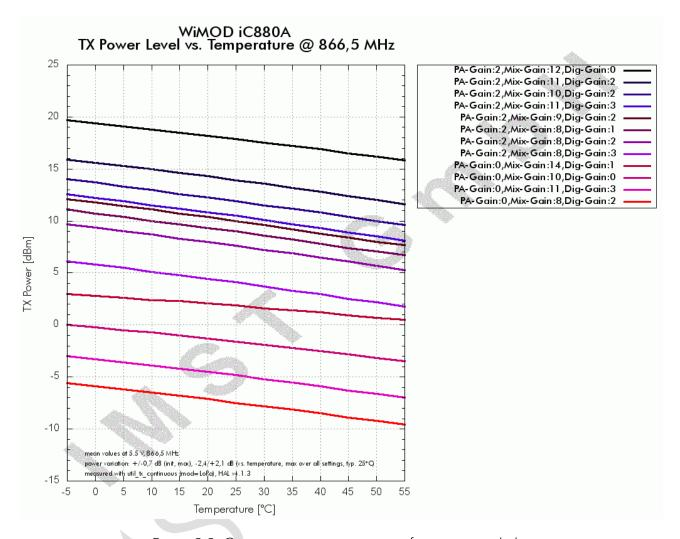
Figure 3-3: Output power vs. temperature for recommended settings
