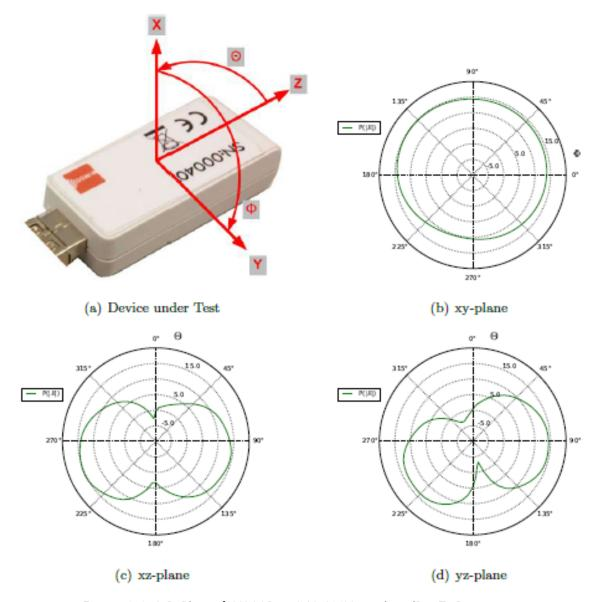
Figure 4-4: 2-D Plots of iU880B at 869.9MHz and 15dBm Tx Power
