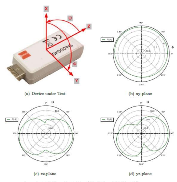
Figure 4-3: 2-D Plots of iU880B at 866.5MHz and 15dBm Tx Power
