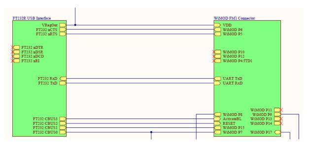
Figure 4-1: Connection between FTDI and iM880B.
