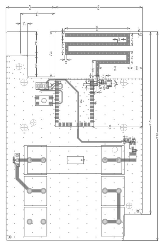
Figure 7-2: Dimensions (in mm) of the antenna
