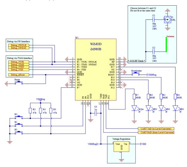
Figure 7-3: Typical Application Schematic for iM980B-MBand
