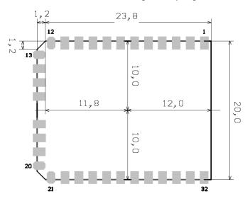
Figure 5-2: Outer Dimensions of the iM980B-MBand (top view)
