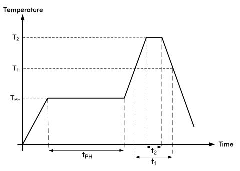
Figure 7-4: Soldering Profile
