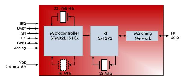
Figure 2-1: Block Diagram of Radio Module iM980B-MBand
