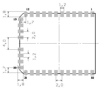
Figure 5-3: Recommended footprint of the iM980B-MBand (top view)
