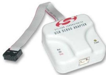
Figure 2-1: Silicon Labs programming adapter
