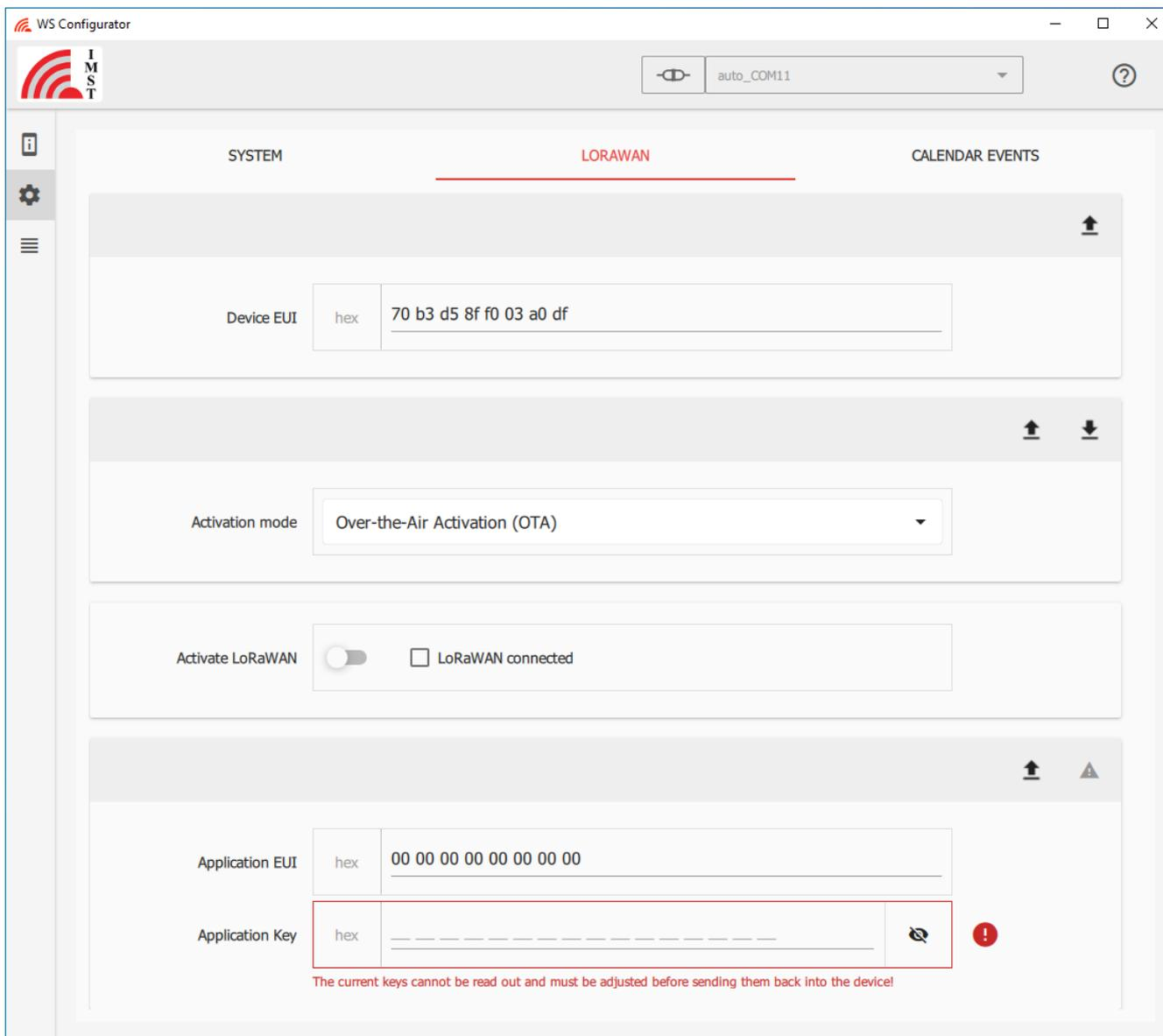
Now a first test if the network can be reached by iO881A can be started. Therefore start the activation of the LoRaWAN stack by moving the slide switch to the right side. iO881A then starts the joining procedure. You can check either on the network server side if the corresponding "Join Requests" are received by the network server or observe the LED signalling of iO881A.
