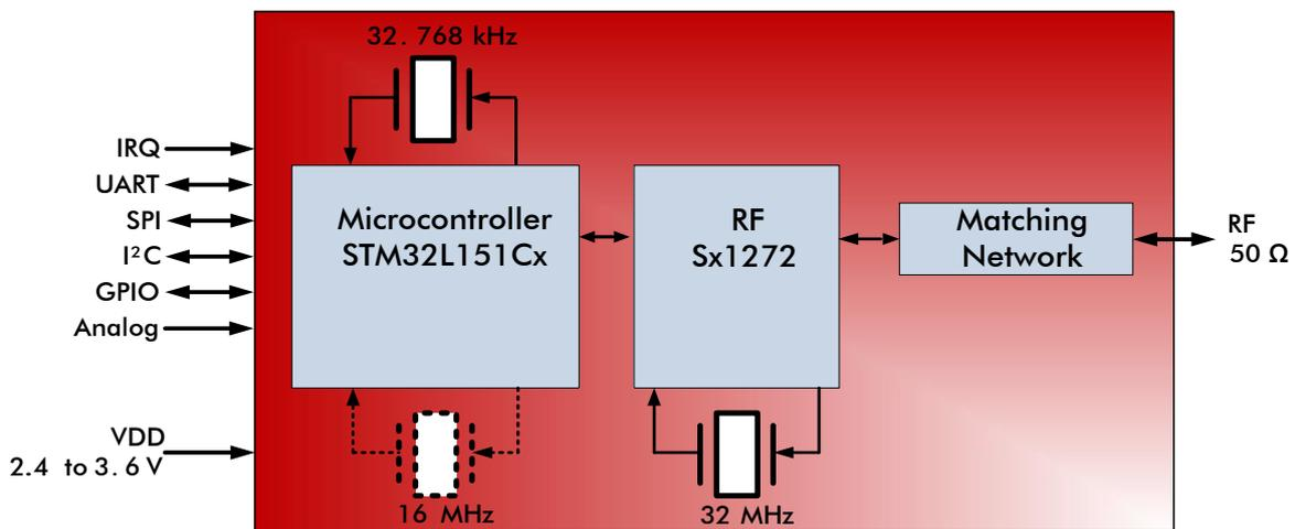
Figure 2-1: Block Diagram of Radio Module iM980B-MBand
