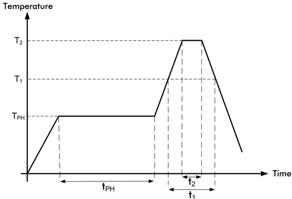
Figure 7-4: Soldering Profile
